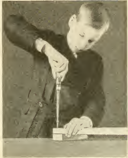
Fig. 14. Proper Position to Hold Screw Driver
